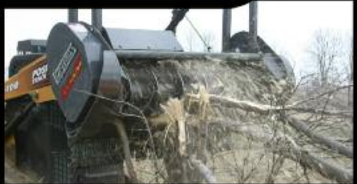
Kwik AX - Downward Rotating "Ax" Type Blades
