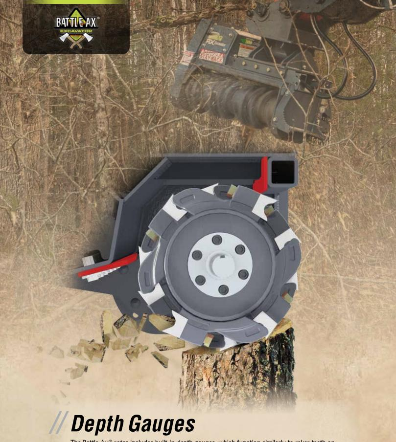
The Battle Ax® rotor includes built-in depth gauges, which function similarly to raker teeth on chain saws to prevent the attachment from engaging too much material at one time. This unique design is more ideal for managing the amount of material being fed into the attachment than competitive ring-style rotors, which many operators find to be overly limiting.
