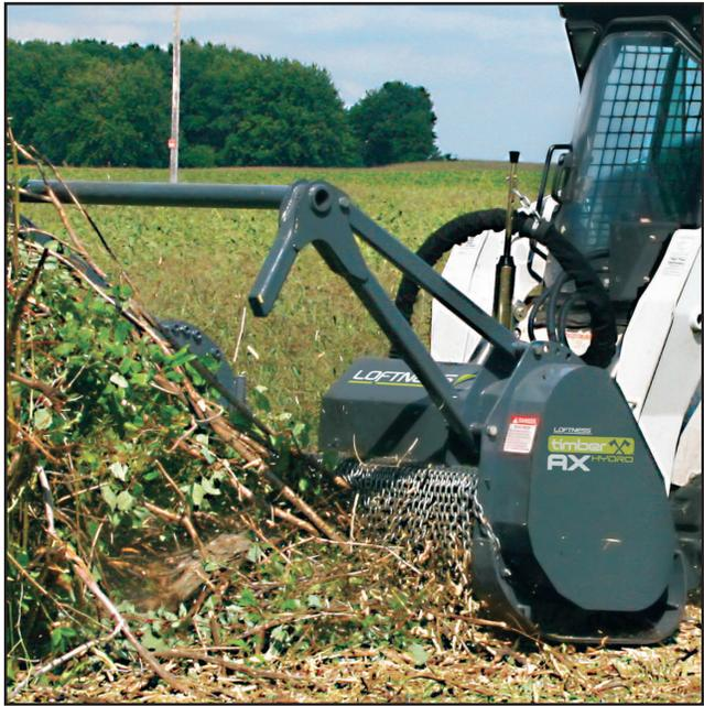
Tilt attachment mounting frame back and raise the Timber Ax slightly above the ground when moving the Timber Ax and machine.
