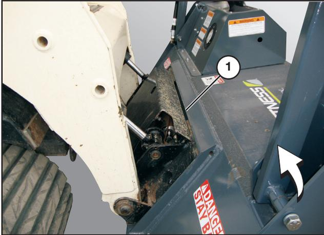
Tilt the loader mounting plate ahead. Drive forward with the loader and hook the top edge of the loader mounting plate under the top flange (1) on the Timber Ax mounting plate. Be careful not to damage the locking levers on the loader mounting plate.
