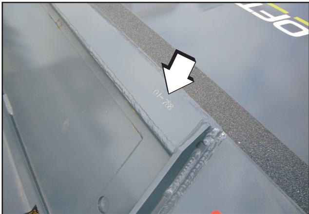
The serial number is also stamped into the frame, on top of the hitch support.
